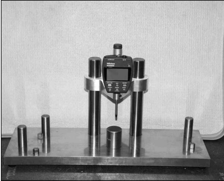
Figure 4. Example of a bow-test rig with a digital gauge and a reference cylinder for zero setting. The reference piece (a cylinder) is preferably made of invar steel and has a height of 30 mm, i.e. the same as the thickness of the specimens.
