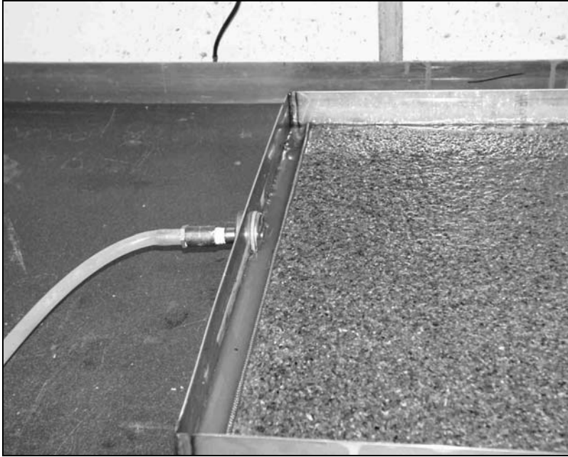
Figure 2 B. Inner pan with sand bed and a water hose. Here complemented with an adjustable water level outlet.
